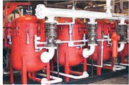
3M high flow liquid filters help maintain water quality in waterflood systems, reducing need for reservoir stimulation.
