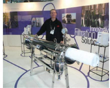
**Paul McNicholas, from 3M, with the 3M High Flow Sanitary Filter Housing. The machine is open to show the single large filter cartridge.**
