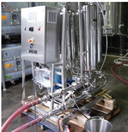
**The Juclas Mastermind automated cartridge filtration system incorporates an automatic back flush and can be used for filtration of still and sparkling wines.**
