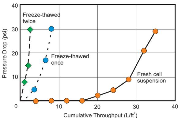
Figure 2 — Filter Throughput vs. Cell Condition
