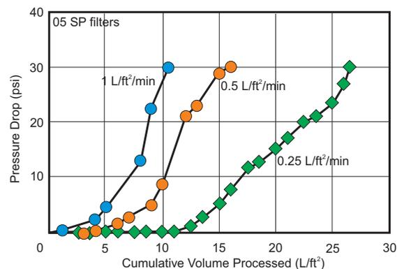
Figure 3 — Filter Throughput vs. Flux Rate
