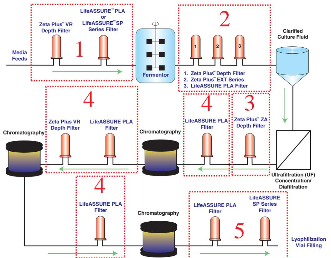
Figure 1 — Typical Manufacturing Process for Ancillary Chemicals
