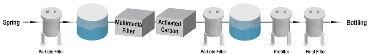
Figure 1 — Typical Spring Water Process'
