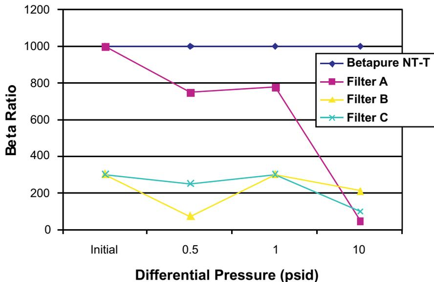
**Filter A: polypropylene gradient pore structure melt-blown filter with core**
