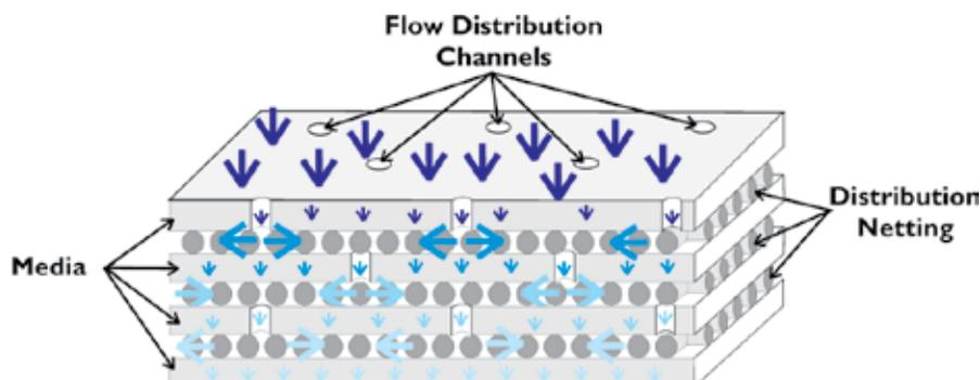
Figure 2 — Betapure NT-T filter media cross-section
