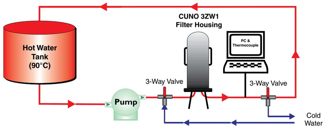
**Figure 4 — Hot Water Test Assembly**
