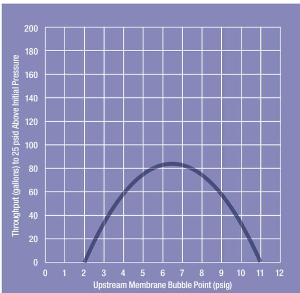
Figure 5. LifeASSURE™ PLA series multi-zone microporous membrane optimization.
