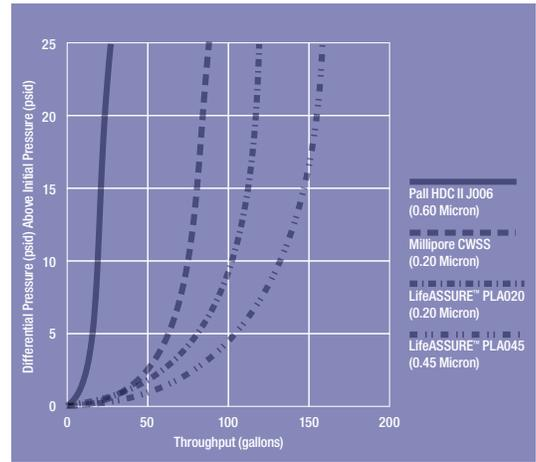
Figure 8. Contaminant capacity of LifeASSURE™ PLA series multi-zone microporous prefilter membranes.
