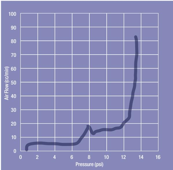
Figure 4. Forward flow bubble point wet in 60/40 IPA/H<sub>2</sub>O.
