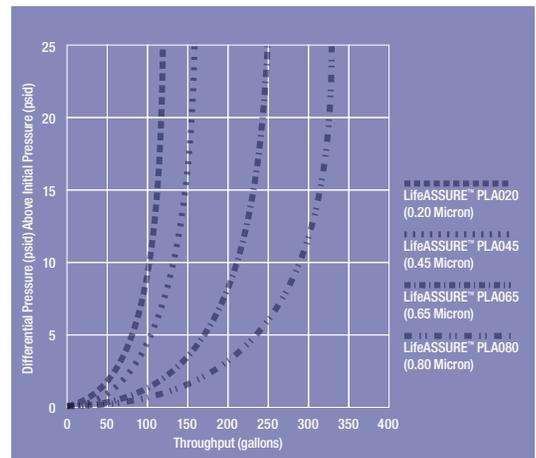
Figure 9. Contaminant capacity of LifeASSURE™ PLA series multi-zone microporous membranes and competitive prefilter membranes.
