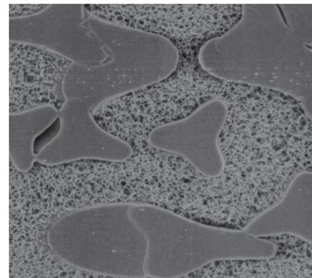
Figure 2. SEM of single zone isotropic membrane.
