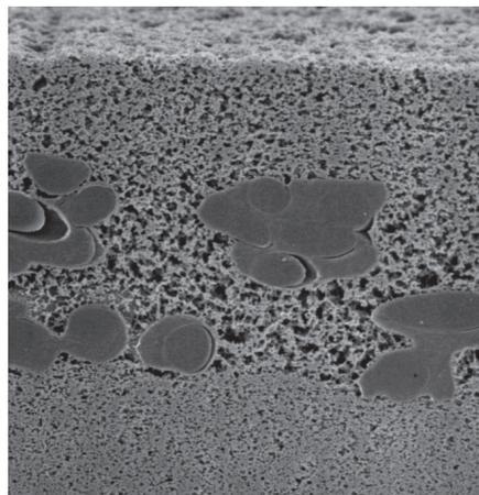
Figure 3. LifeASSURE™ PLA series integral multi-zone microporous membrane.
